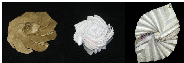
Fig. 1. Example of an origami structure (left) and flasher hat mechanism in its fabricated (middle) and deployed form (right).
